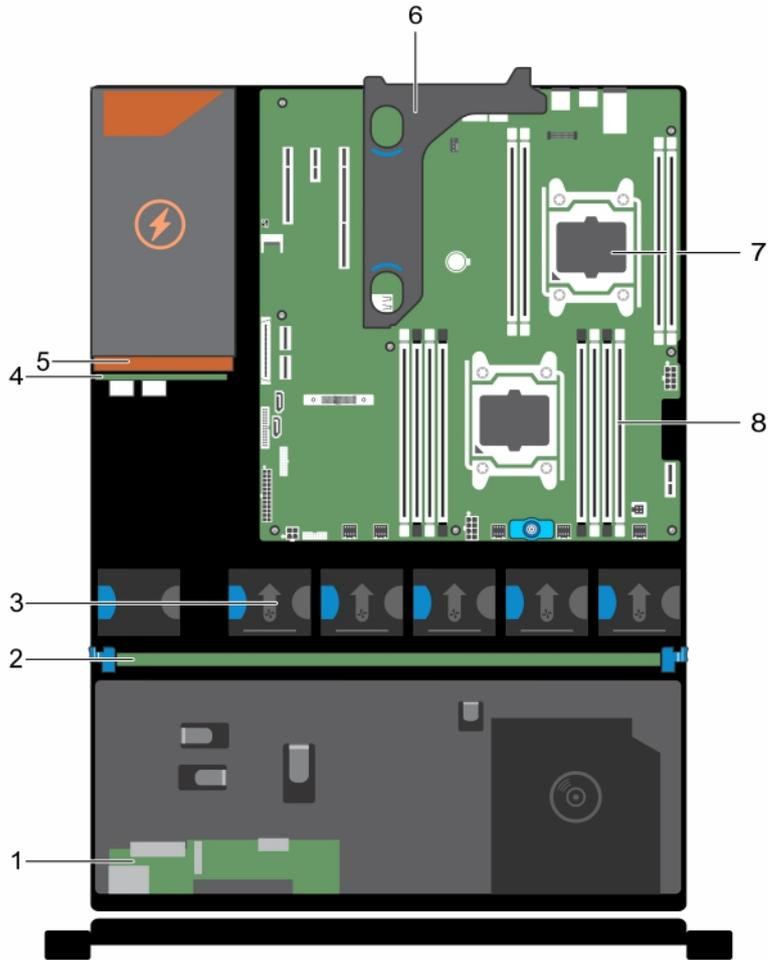
**Figure 11. Inside the System—Redundant Power Supply Unit Chassis**
