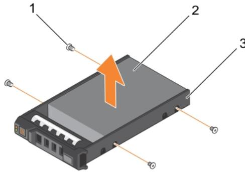
Figure 22. Removing and installing a hard drive into a hard-drive carrier
