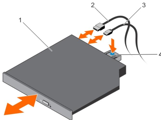
**Figure 23. Removing and installing the optical drive**
