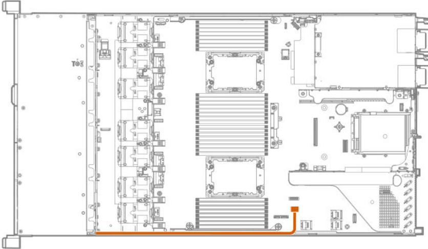
8. Using a Torx T-10 screwdriver, remove the Power/UID/USB assembly.
