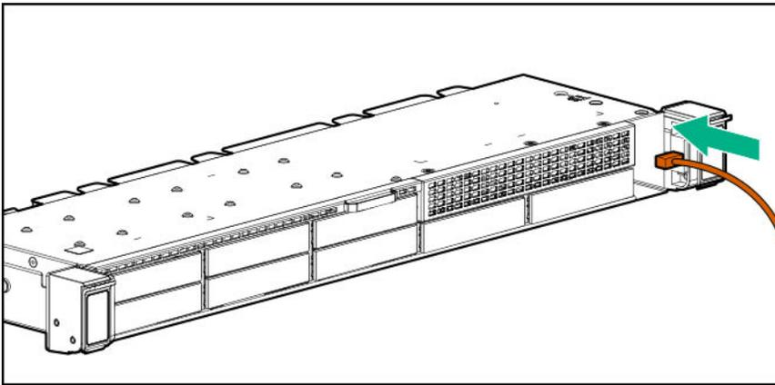
10. Install the SID module into the front panel. Using a T-10 Torx screwdriver, secure the module to the chassis with the screws from the kit.
