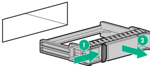
Figure 1: Removing an SFF drive blank
