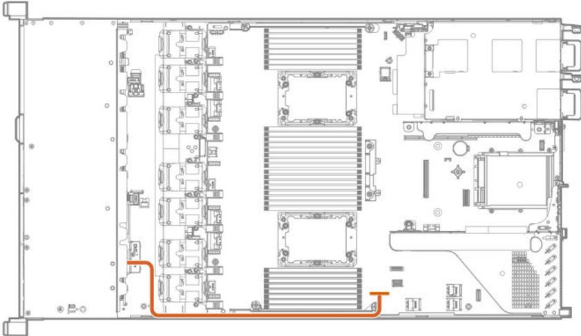
**LFF front display port/USB cabling**
