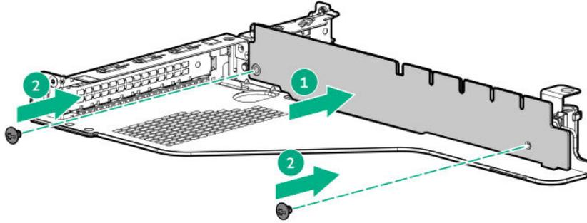
9. Remove the screw securing the standoff on the riser.
