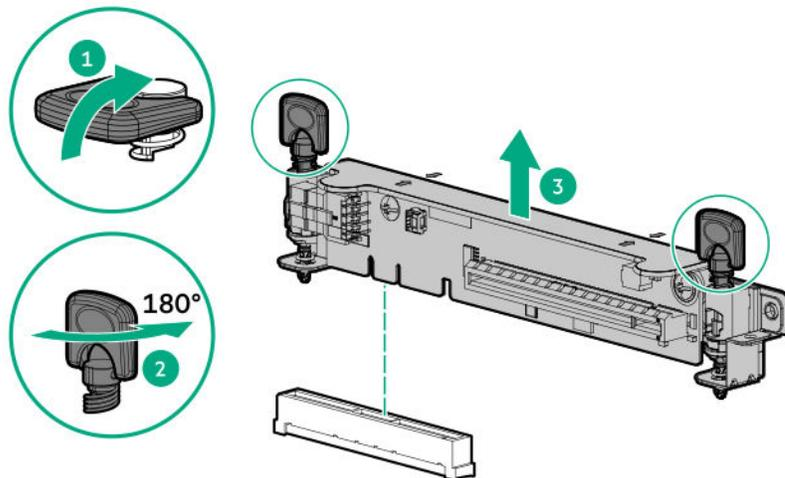
8. Lift and remove the secondary riser cage latch.
