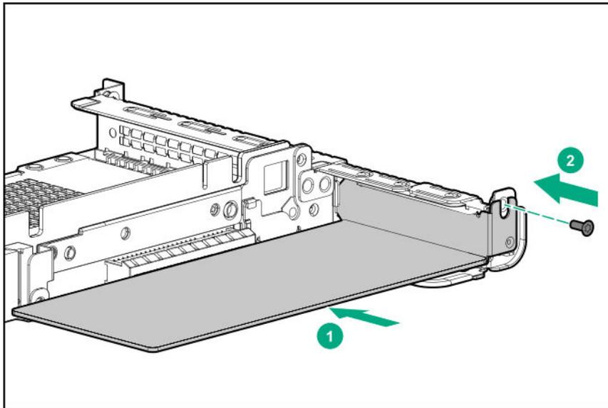
10. Install the PCIe riser cage into the server.
