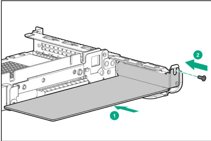
**8. Install the secondary PCI riser cage.**
