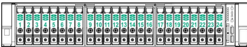
When any stacked 2 SFF drive cage is connected to the SAS expander, the drive numbering skips the second number. For example, when a rear 2 SFF drive cage is connected to SAS expander port 9, then the drive numbers are 25 and 27.
