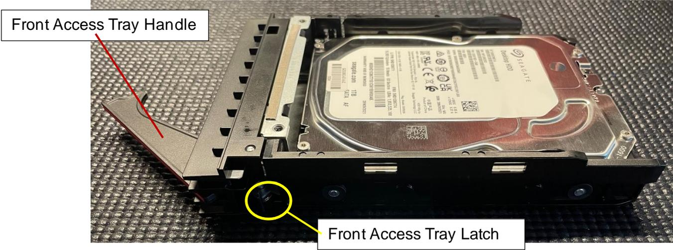
5. Slide the front access HDD tray into the front access bay as shown below.
