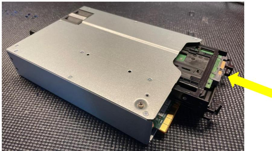
5. Here is what the end of the PSU bay storage enclosure should look like when the drive is fully installed.
