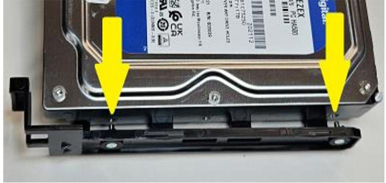
4. Slide the SATA HDD tray back into the PSU bay storage enclosure until it latches into place as shown below.
