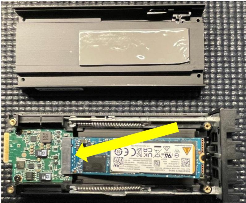
5. Push down on the M.2 drive and install the screw used to secure the M.2 drive to the M.2 carrier.
