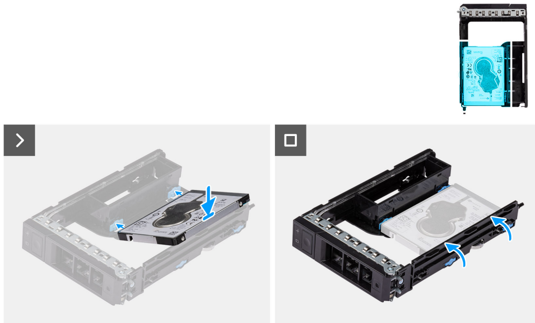
Figure 24. Installing a 2.5-inch hard drive from the external hard-drive assembly
