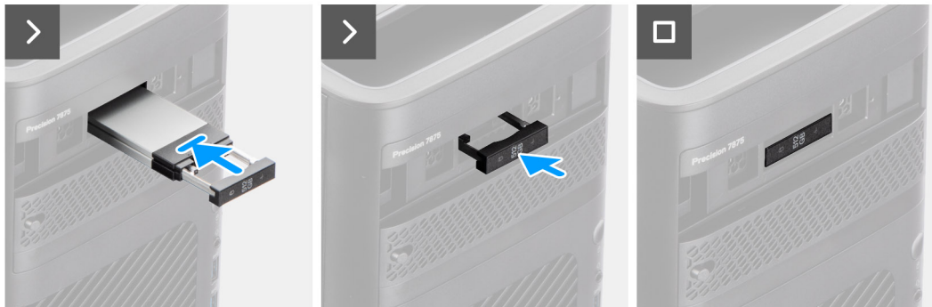
Figure 37. Installing the external solid-state drive assembly
