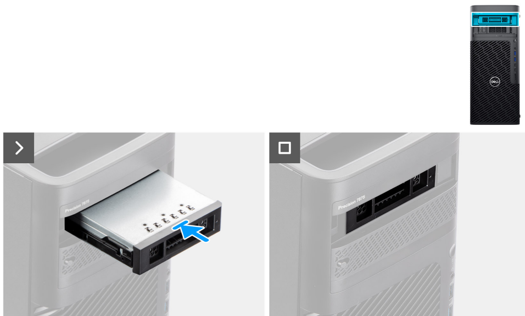
Figure 31. Installing the external solid-state drive cage
