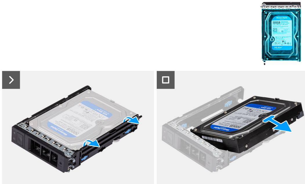
Figure 27. Removing a 3.5-inch hard drive from the external hard-drive assembly
