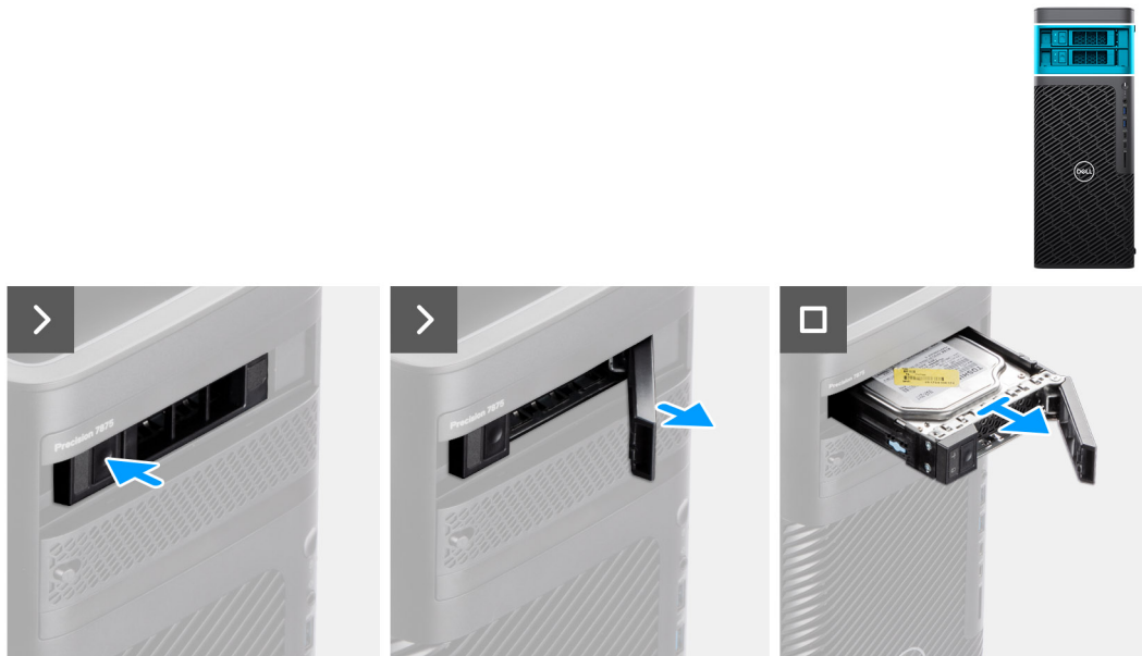
Figure 26. Removing the external 3.5-inch hard-drive assembly
