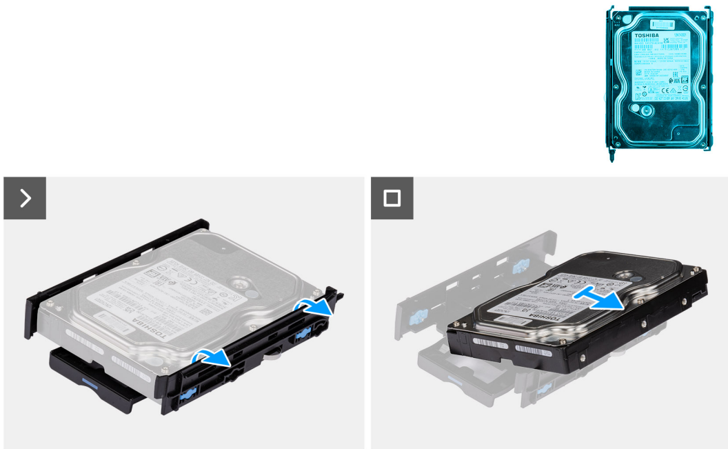
Figure 47. Removing the 3.5-inch hard-drive bracket
