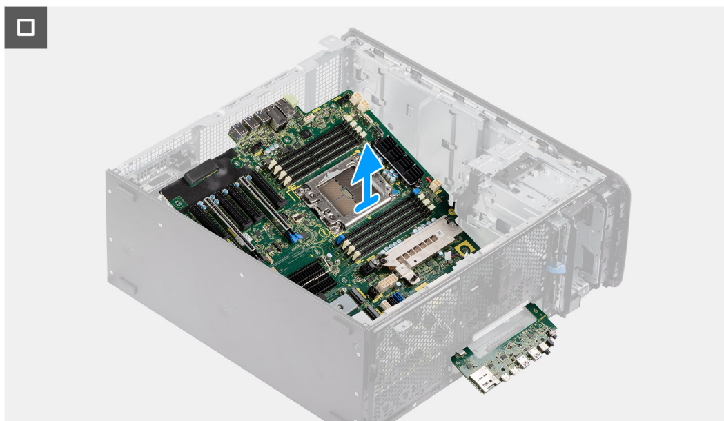
Figure 119. Removing the system board
