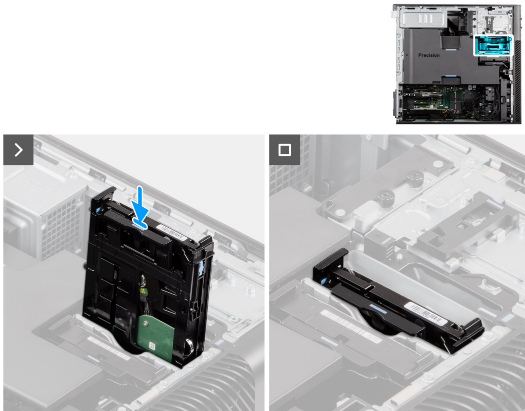
Figure 49. Installing the 3.5-inch hard-drive assembly
