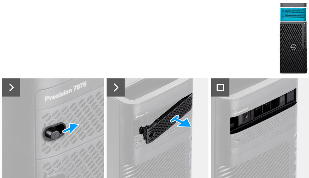
Figure 18. Removing the front bezel with hard drive
