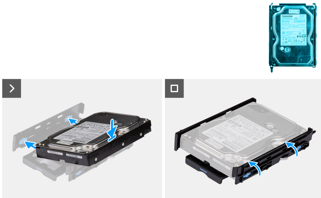
Figure 48. Installing the 3.5-inch hard-drive bracket
