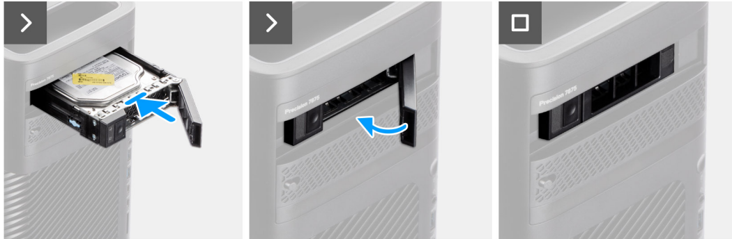
Figure 29. Installing the external 3.5-inch hard-drive assembly
