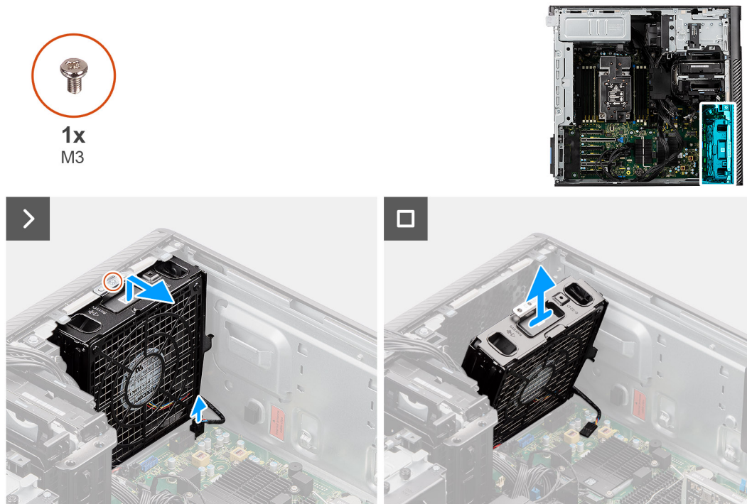
Figure 44. Removing the front-fan assembly
