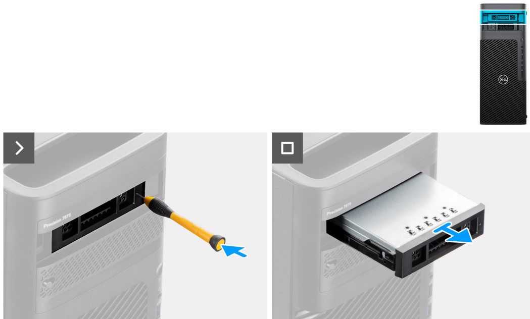
Figure 30. Removing the external solid-state drive cage
