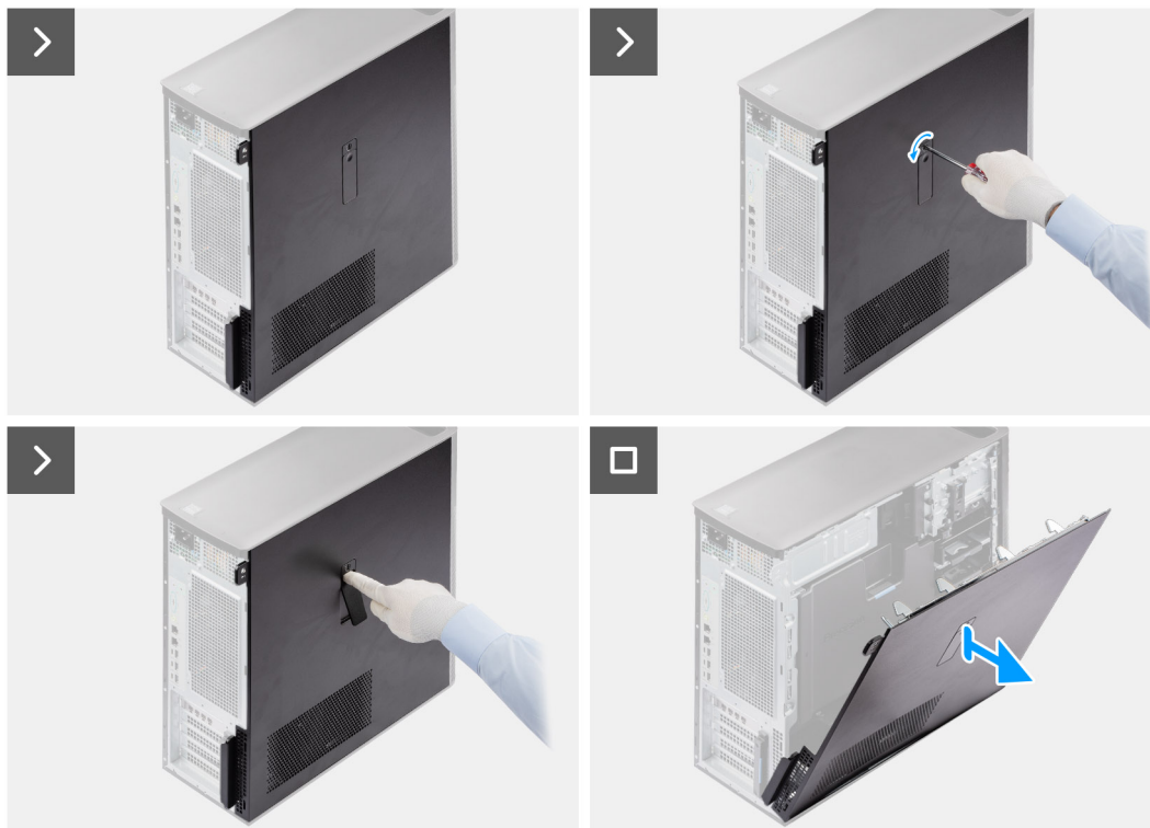
Figure 10. Removing the side cover
