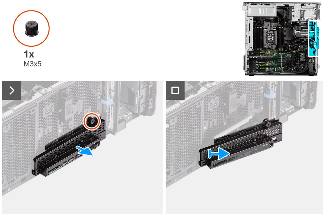
Figure 16. Removing the front I/O bracket
