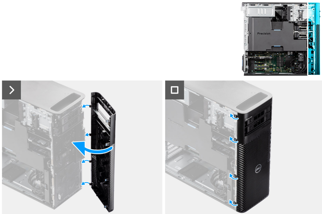
Figure 13. Installing the front bezel
