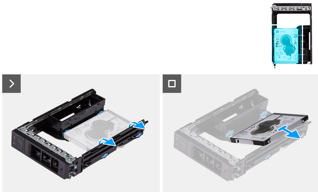
Figure 23. Removing a 2.5-inch hard drive from the external hard-drive assembly
