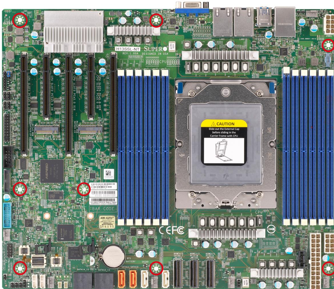
Figure 2-1. Motherboard Mounting Holes
