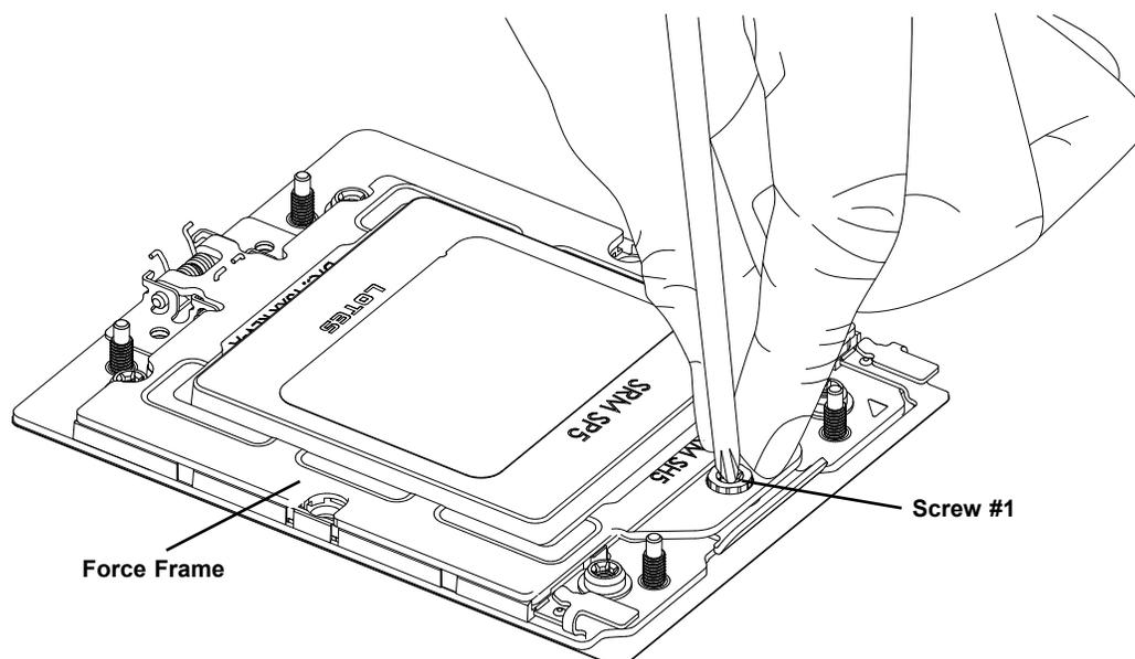
2. The spring-loaded force frame will raise up after the screw securing it (#1) is removed. Gently allow it to lift up to its stopping position.
