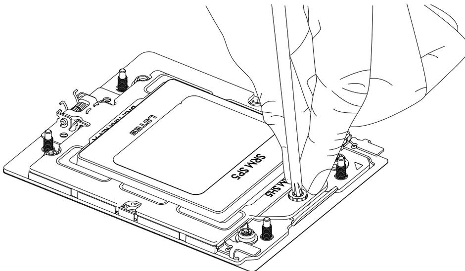
10. Replace and tighten the screws in the same order you removed them. When finished, the force frame will be secure over both the rail frame and CPU package.
