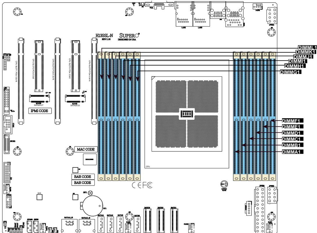
Figure 2-2. DIMM Numbering
