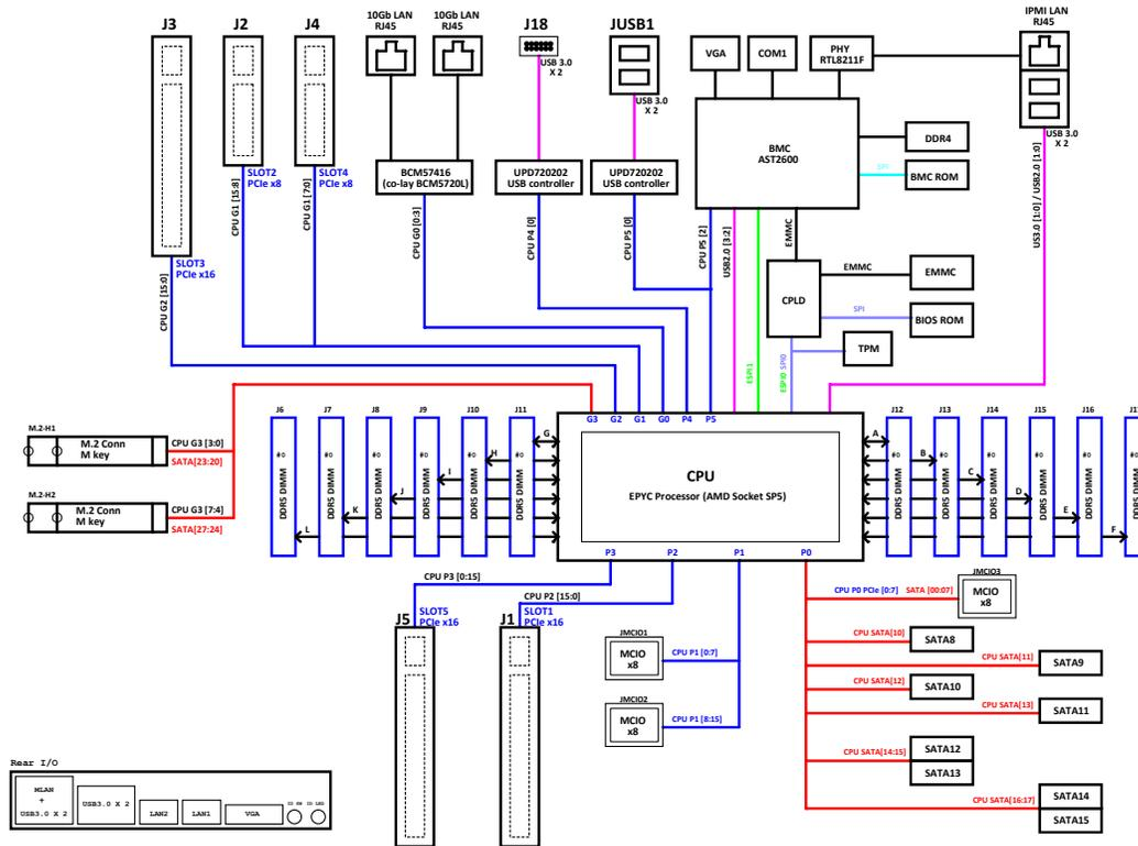
Figure 1-4. System Block Diagram
