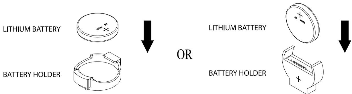
**Figure 3-1. Battery Installation**
