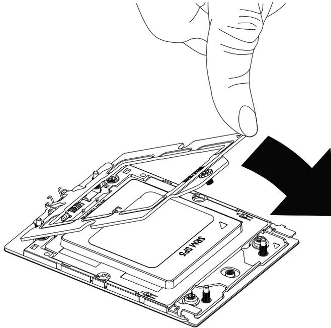
9. The force frame is spring loaded and has to be held in place before it is secured.
